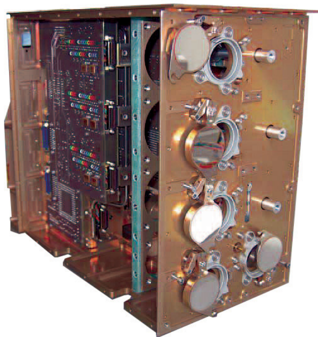
Figure 1. The PREMOS experiment partly assembled. Filter radiometers are behind the upper three covers and two absolute radiometers are in the lower part of the instrument.
